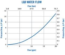
These graphs are intended to give you a general idea of the performance capabilities of each product line. Contact CPC for flow of a particular coupling combination.
